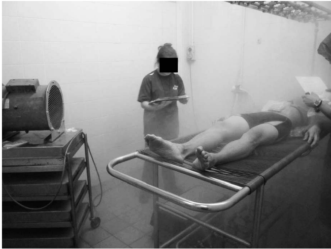
Figure 1. Body-cooling unit. Ambient-temperature water dispensed as a fine mist from pressure valves above and below the participant with a fan blowing across participants from feet to head. The unit is similar to a misting fan except that it dispenses mists of water from the bed rather than from the fan.
