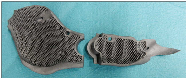
Figure 3: Medial part of a left-sided jaw border implant in two parts with a large three-dimensional puzzle design. Each part has two holes for screw fixation. The scaffolding is clearly visible
