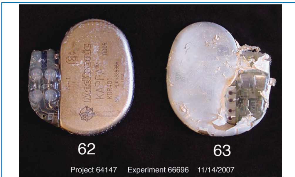
Figure 8. Representative biofilm formation at 7 days on pacemakers with or without the AIGISRx™ envelope after implantation in a rabbit model of infectivity using Acinetobacter baumannii . Left: with AIGISRx™ envelope; right: without AIGISRx™ envelope (Hansen et al. 33 by permission).
