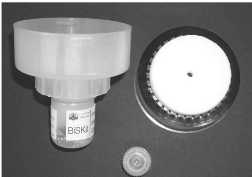
FIG. 1. BiSKit. The components include a BiSKit sampling unit, a 30-ml sample collection bottle with buffer, a dropper attachment, and a rubber cap.
