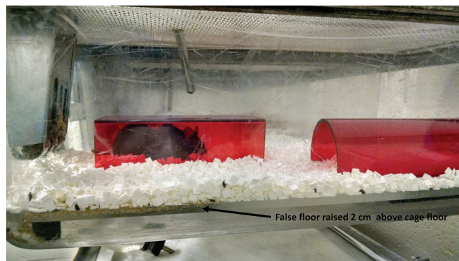
Figure 4. Photograph of 2 female C57BL6 mice huddled together in a heated refuge consisting of a red hut placed over an active plate in a standard cage with ALPHA-dri bedding (Shepherd Specialty Papers, Watertown, TN). The hut to the right sits over an inactive heating plate.
