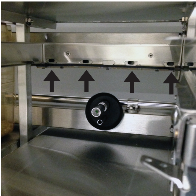
Figure 3. Horizontal exhaust air ports located at the rear of the cage slot (arrows) draw the cage-exhausted air into the horizontal exhaust plenum on an IVC rack (Allentown, Allentown, NJ).
