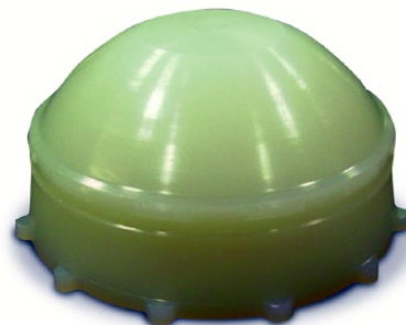
Fig. 2 Highly crosslinked polyethylene insert treated with vitamin E.
