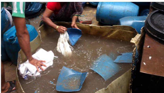
Figure 5 Women plastic workers with no protective equipment rinse plastic materials in acid.
