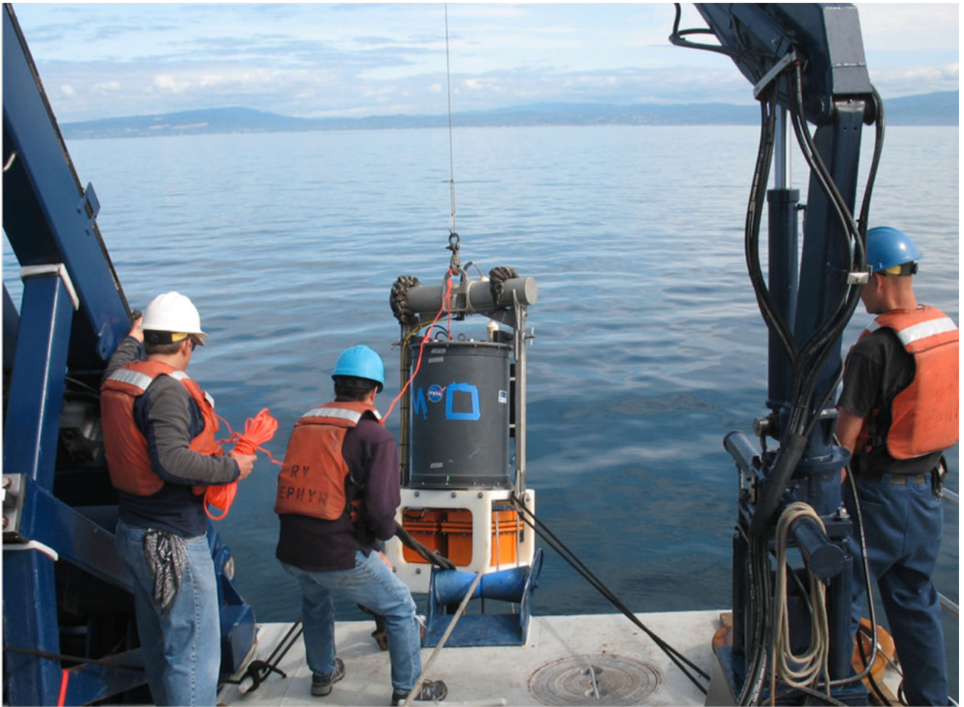
Fig. 6. The Environmental Sample Processor (ESP), a device developed for in situ automated detection of HAB species and toxins (Source: C. Scholin, Monterey Bay Aquarium Research Institute).
