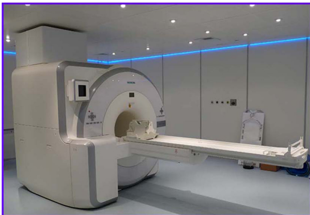
Fig. 13 The combined PET/MR scanner (Siemens Healthineers) with simultaneous MR and PET imaging capability.
