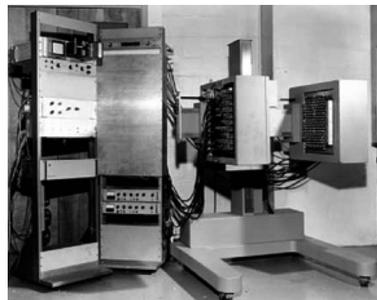
Fig. 2 One of the first positron imaging devices, the positron camera that was developed by Dr. Brownell and his team at Massachusetts Hospital (MGH) in Boston. The device became operational in 1969 and consists of two planar arrays of crystals. The patient is positioned between the two detectors.
