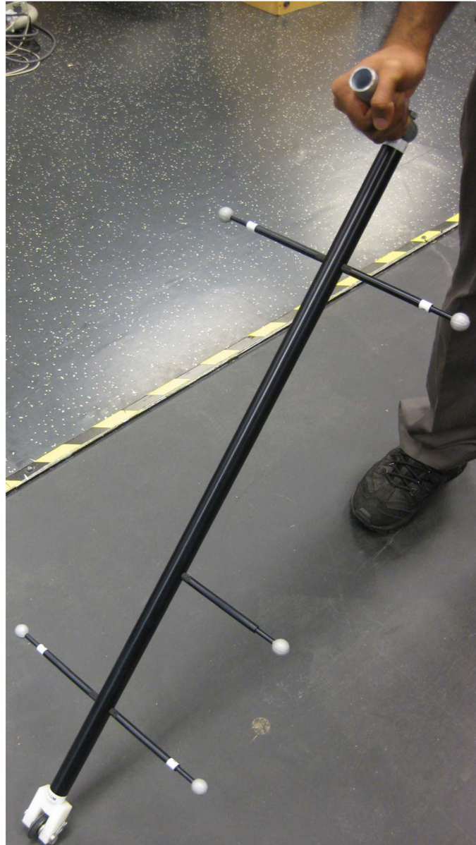
Figure 3. Custom rolling digitizing wand based on CalTester.
