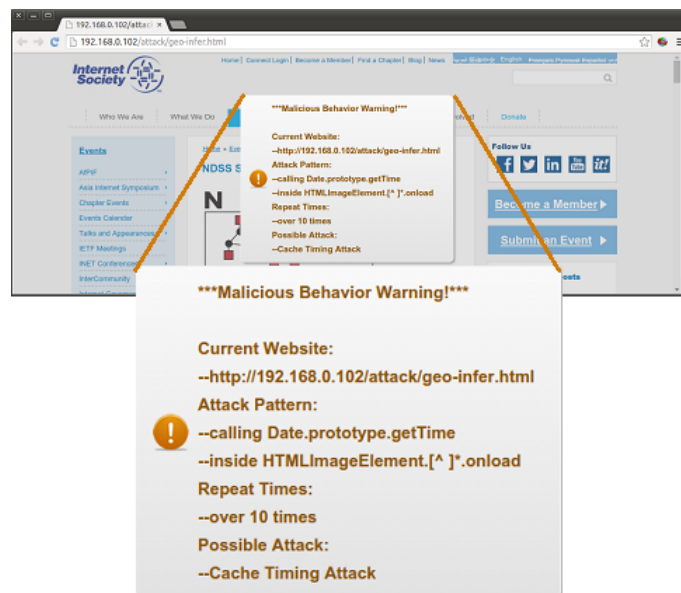
Figure 5. Given a malicious website, once the probing behavior detector finds suspicious behaviors, it raises an alert to warn the user.
