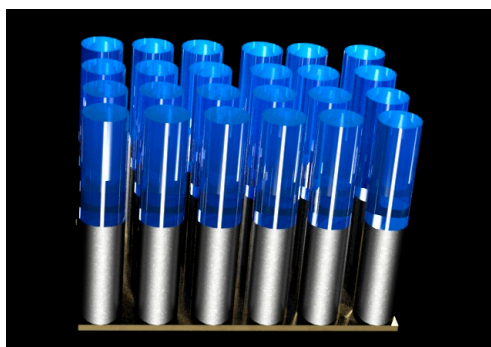
Figure 7. Schematic illustration of Au-PPy nanorods.
