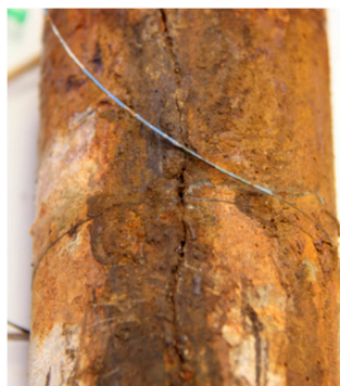
Figure 11. Illustration of cracking of the specimen.
