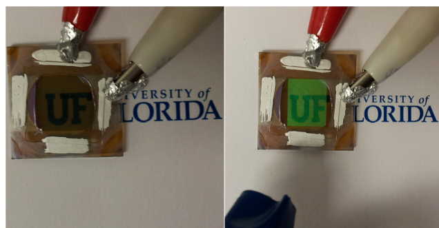
Figure 4 | Images of transparent IR sensitive OLED. Images of a transparent IR-OLED with a PbS IR sensitizer operated in ambient light (left) and under IR illumination (right).
