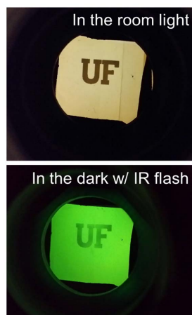
Figure 5 | Demonstration of pixelless IR imaging. The photo images of the pixelless IR imaging demonstration by a monocular direct view IR imager fabricated with a transparent IR sensitive OLED under room light (top) and in the dark with the 1.2 \mu\text{m} IR flash light (bottom).
