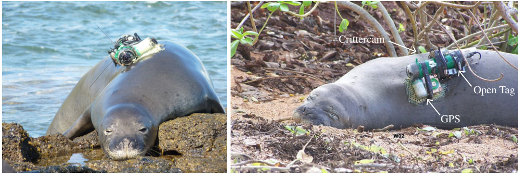
Figure 2. Photo of the instrument package attached to a Hawaiian monk seal. The package includes a National Geographic Crittercam, a Loggerhead Instruments Open Tag and a SMRU GPS phone tag.
