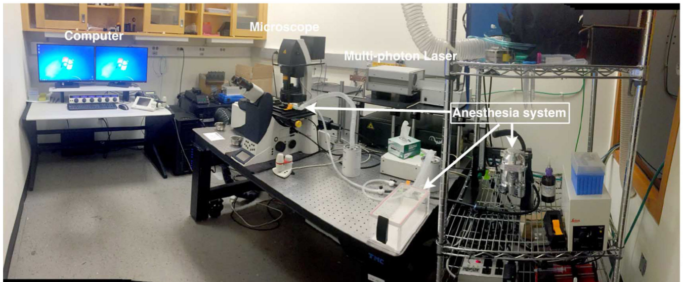
Figure 1. Inverted Multi-photon setup
