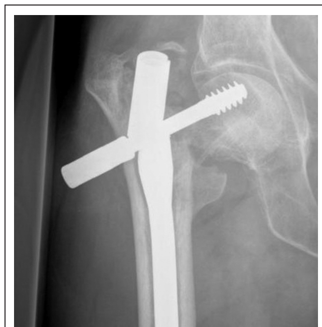
Figure 1 Anteroposterior radiograph showing fracture of nail through barrel lag screw aperture
