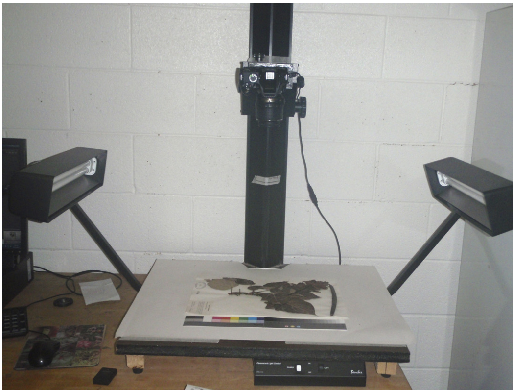
Fig. 2. The imaging station at the Arkansas State University (STAR) Herbarium that was assembled from existing herbarium resources and purchased materials. The figure shows the fluorescent sidelights, the Nikon D3200 camera, the color separation guide and ruler (purchased for the project), and the Bencher Copymate II copy stand (previously existing in the herbarium). The total new cost for the set-up was approximately US$1500.
