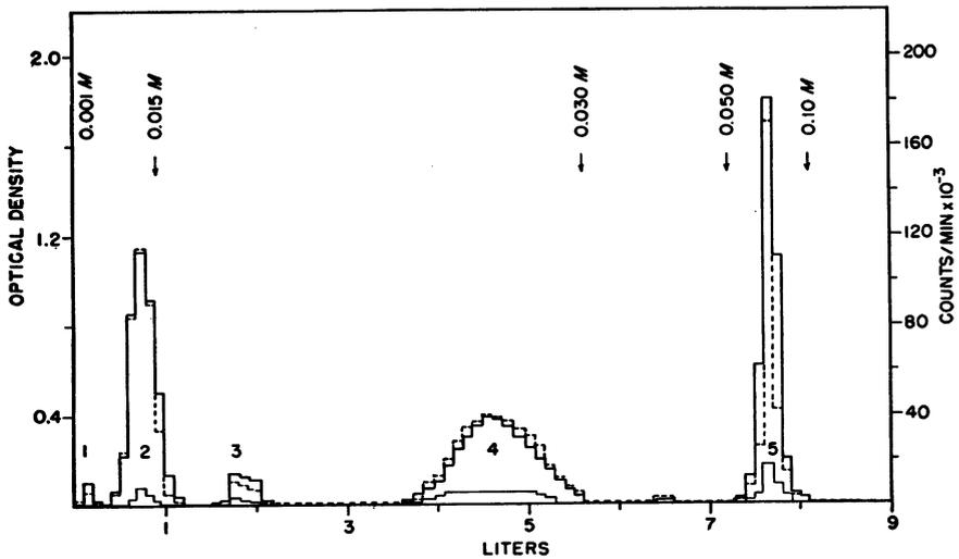
FIG. 1. Separation of the sugars in *Phytolacca decandra* by ion-exchange chromatography of their borate complexes. Resin bed, 0.85 sq. cm.  $\times$  12 cm.; Dowex-1 resin (200–400 mesh), borate form. Elution started with 0.001 M potassium tetraborate, changed to 0.015 M at 900 ml., to 0.030 M at 5600 ml., to 0.050 M at 7200 ml., and to 0.10 M at 8100 ml.
