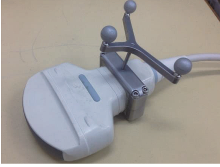
FIGURE 2: A DRF set on an ultrasound probe.
