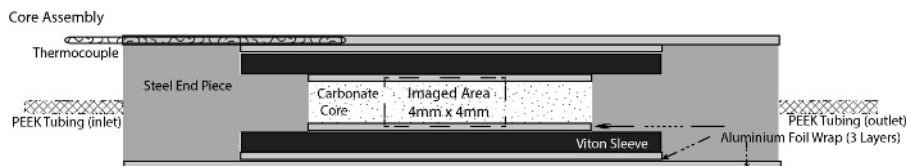
Figure 4. The core assembly inside the core holder. PEEK tubing is attached to the interior end fittings and threaded through the steel end caps. The core is wrapped in aluminum foil and inserted into the sleeve. The sleeve is then stretched over the end fittings to create a watertight seal and two additional layers of aluminum foil are added to hold everything in place and prevent gas diffusion. The thermocouple is secured to the outside of the core assembly with the outer layer of adhesive aluminum foil. Figure modified from Menke et al. 42 . Please click here to view a larger version of this figure.
