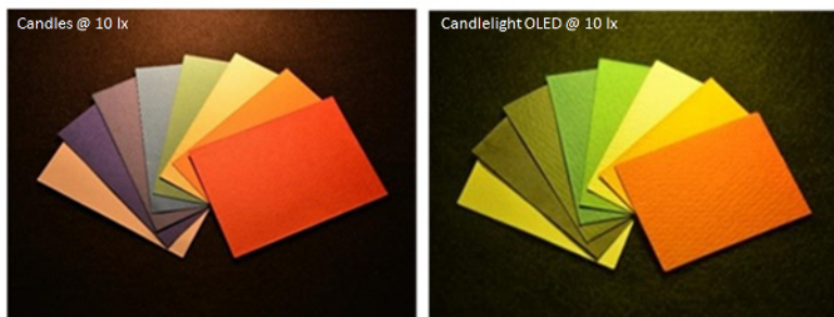
Figure 5: Photographs of cloud papers with rainbows and white colors illuminated by candles (left) and a blue-hazard-free candlelight OLED (right) at 10 lx 34 . Please click here to view a larger version of this figure.
