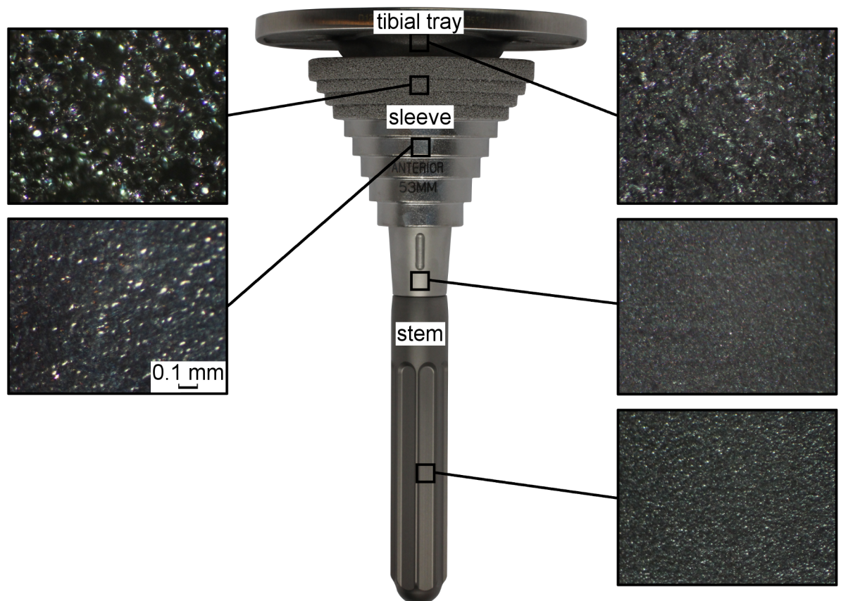
Fig 2. Microscopic and macroscopic surfaces of a tibial tray, combined with sleeve and distal stem.
