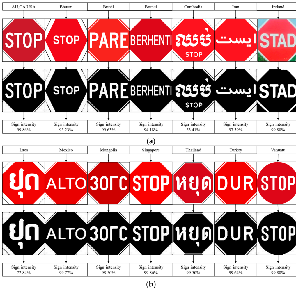
Figure 23. Robustness testing, (a) Seven set of different countries' stop sign; (b) Seven sets of different countries' stop signs.
