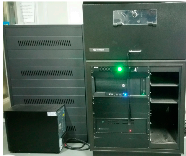
Figure 9. Nano-indentation film test system.
