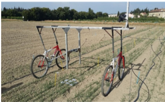
Fig. 1 The moving platform used to take the images in the field in 2014
