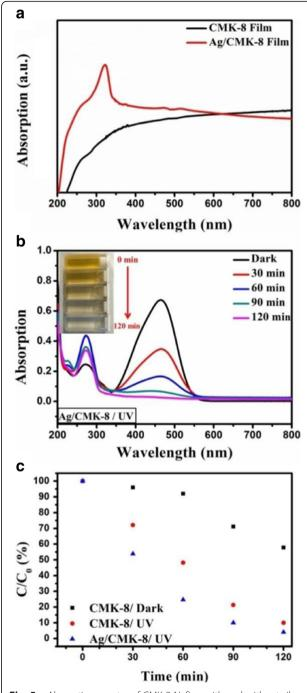
**Fig. 5 a** Absorption spectra of CMK-8-Nafion with and without silver NPs. **b** UV-Vis spectrum evolution of MO decomposition with the Ag/CMK-8-Nafion membrane. **c** A comparison of MO decomposition efficiency levels with different experimental conditions
