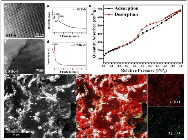
Fig. 1 Characterization of KIT-6 and corresponding CMK-8. a, b High-magnification TEM images. c, d Small-angle XRD patterns. e N<sub>2</sub> adsorption/desorption isotherms (77 K) of CMK-8. f, g SEM image and corresponding EDX elemental mappings of C, Aq, and Ag/CMK-8-Nafion membranes
