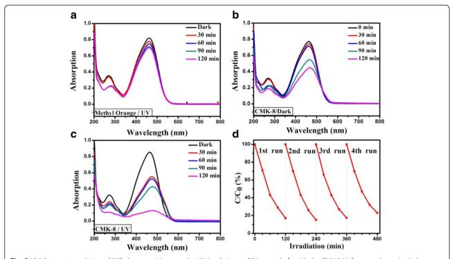
**Fig. 3** UV-Vis spectra evolution of MO decomposition **a** under UV irradiation at 254 nm only, **b** with the CMK-8-Nafion membrane in darkness, **c** CMK-8-Nafion membrane under UV irradiation at 254 nm, and **d** recycling examination
