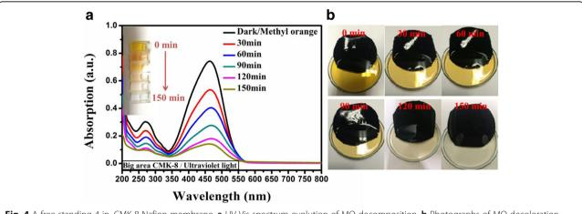
Fig. 4 A free-standing 4-in. CMK-8-Nafion membrane. a UV-Vis spectrum evolution of MO decomposition. b Photographs of MO decoloration under UV irradiation at 254 nm
