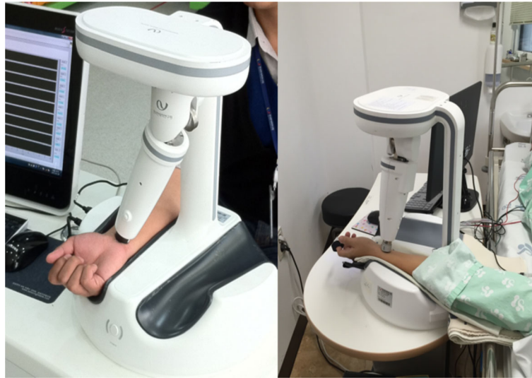
Fig. 2 The overall features of KIAM-PAS for the assessment of radial artery pulse pressure in different positions ( left : sitting position, right : lying position). The figure was epitomized from the previous article that described the study protocol of this study [11]
