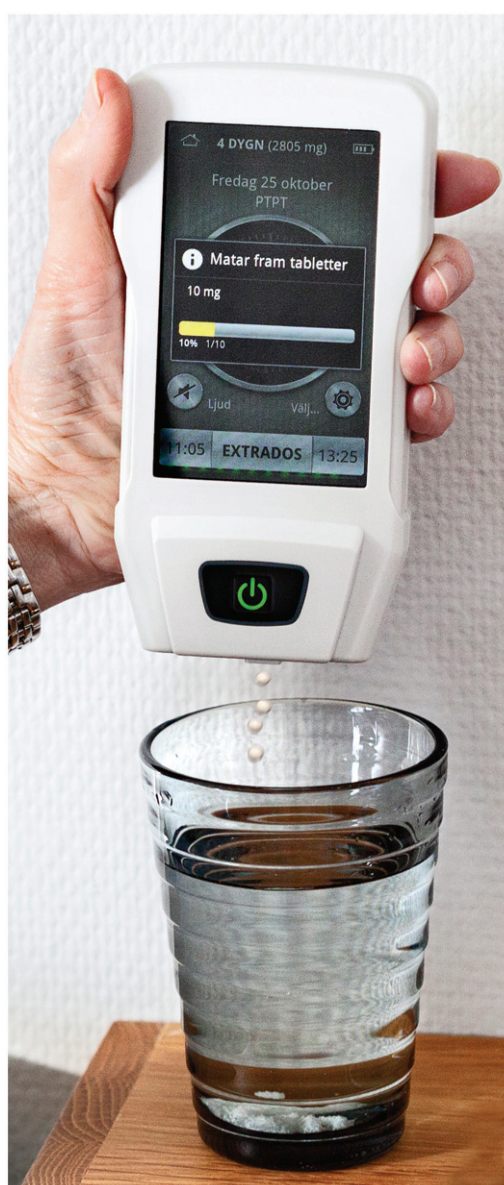
Figure 3. Automatic dose dispenser for levodopa/carbidopa microtablets.
