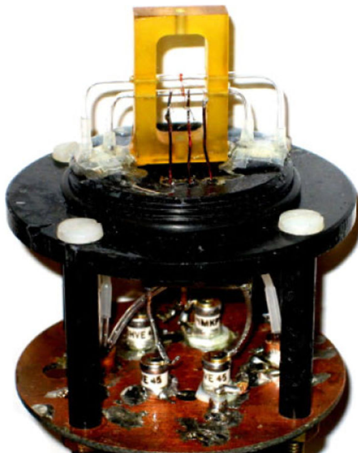
Figure 1. Microcoil difference probe head displaying sample capillaries and sample coils. The rest of the resonant circuitry is located just below the sample cells.
