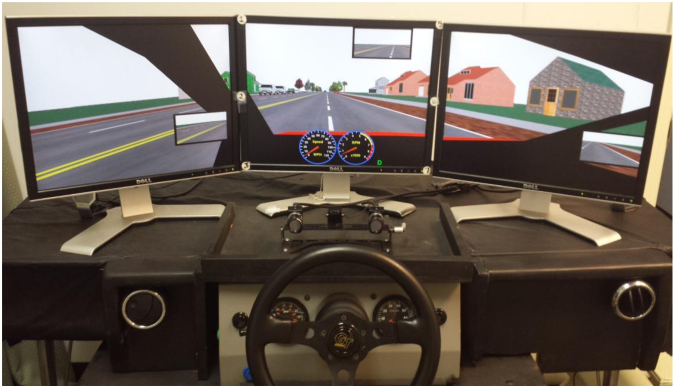
Figure 1. STISIM driving simulator
