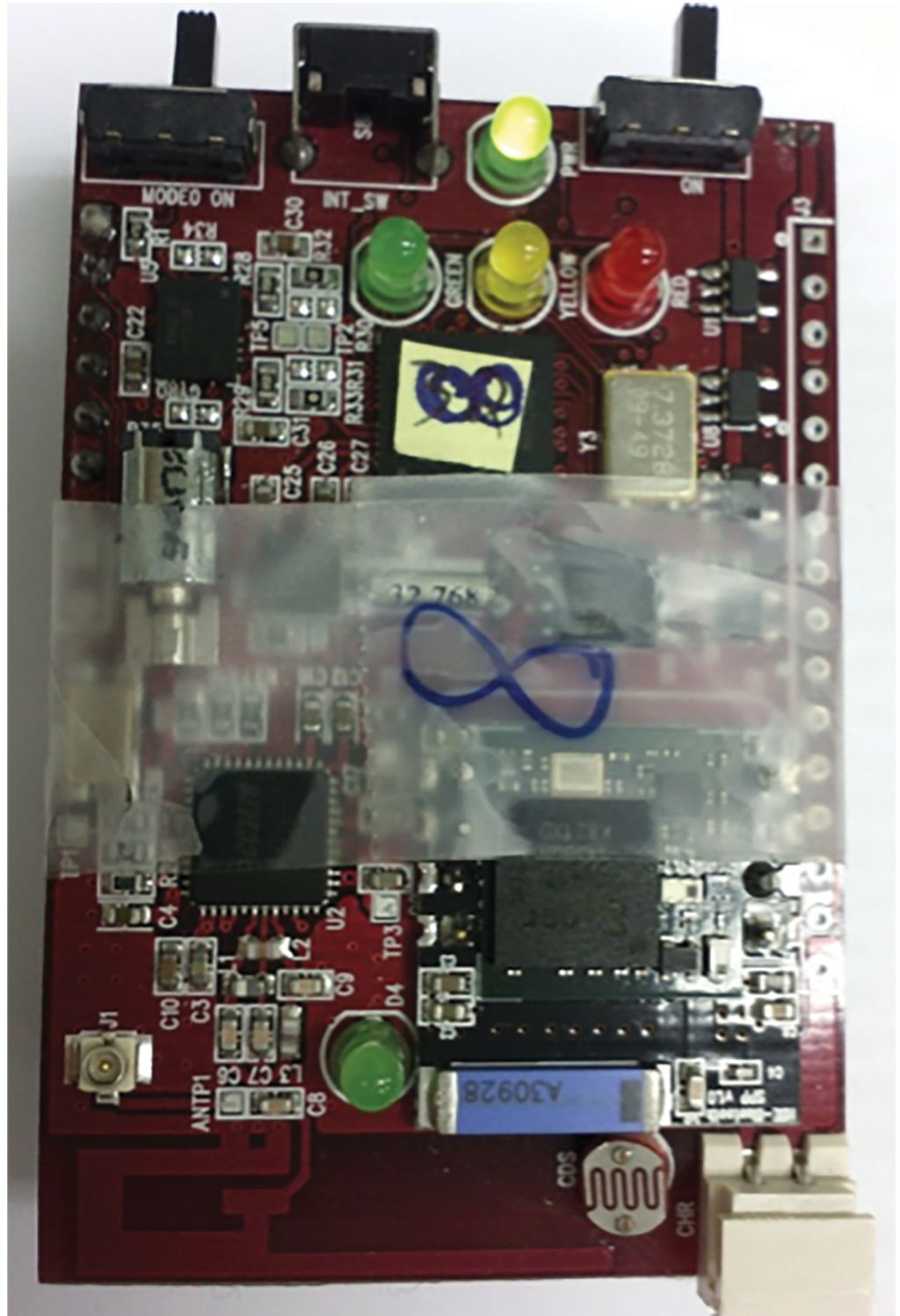
Fig 2. Portable radio signal strength indicator device used to measure radio signal strength from other devices. Social event participants wore necklaces carrying the devices.
