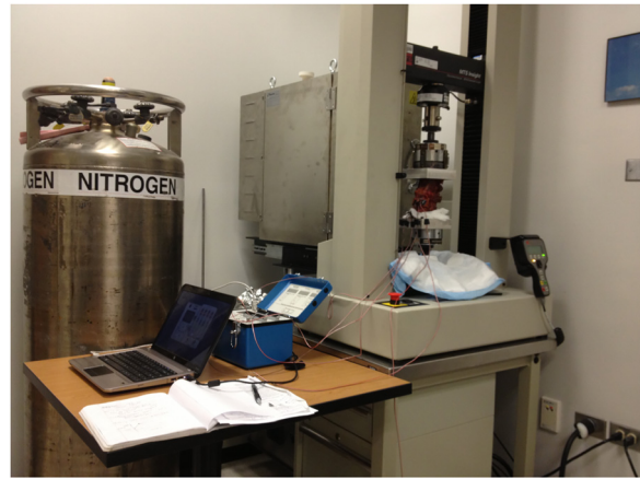
Fig. 3 Experimental setup. Compressive loads were applied to the L4–L5 unit via compression platens with the proximal and distal ends potted in urethane blocks. Strains were measured during loading using a strain recorder and stored on a PC for analysis.
