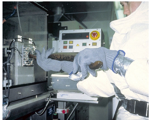
Figure 9: The release of sterilized males has been developed as a potential environmentally benign, species-specific sea lamprey control tactic. The technique requires a dedicated facility and auto-injector (pictured) due to the mutagenic properties of the sterilant P, P-bis (1-aziridinyl)-N-methylphosphinothioic amide (Bisazir). Photo credit: Great Lakes Fishery Commission.
