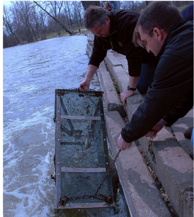
Figure 8: Most purpose-built sea lamprey barriers have adult sea lamprey traps either integrated into their design (top; left side of barrier) or placed along their face (bottom). Although reproductive potential in a stream can be reduced by removing captured adults, high fecundity and compensatory mechanisms prevent significant impact to the recruitment of parasitic juveniles to the lakes. Trapping does serve as a critical assessment tool and holds high promise as a future control technique if tactics that increase trapping efficiencies are developed. Photo credits: Top—M. Ryan, Great Lakes Fishery Commission; bottom—A. Muir, Great Lakes Fishery Commission.
