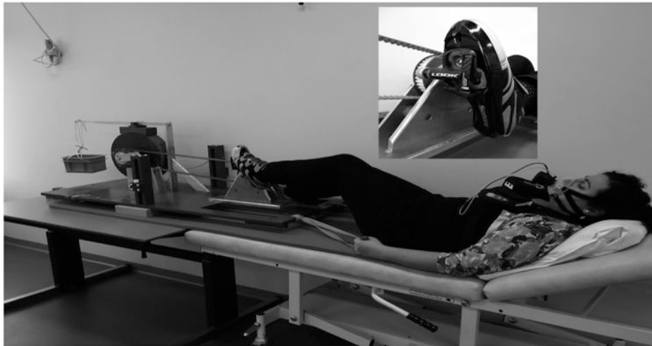
Figure 1. Test subject performing CPET test on the MR-compatible bicycle ergometer in the exercise Laboratory.
