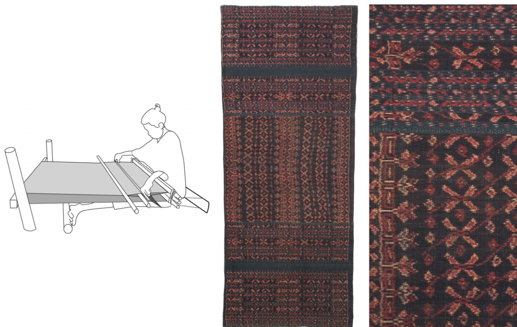
Figure 1. A simple, ground-level loom from Nggela in Flores (Ende Regency), used to weave ikat-decorated cotton sarongs such as the one shown to the right of the loom (whole sarong, detail of ikat decoration).
