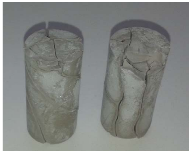
Figure 8. Specimens 1.90 after 40 days exposure to ambient conditions.
