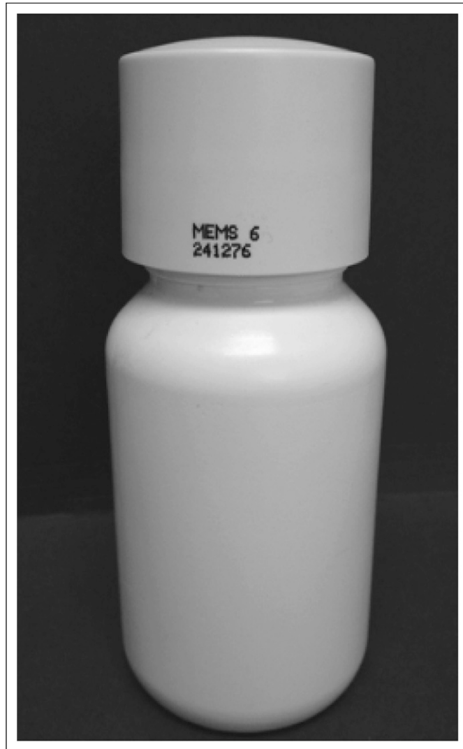
Fig A1. Medication Event Monitoring System (MEMS) pill bottle and TrackCap.
