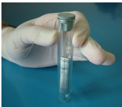
Figure 4. Specimen in glass container suspended on a nylon thread.
