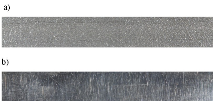
Figure 2. DMLS specimen: (a) before polishing; (b) after polishing.
