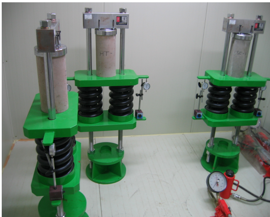
Figure 4. Creep test setup.
