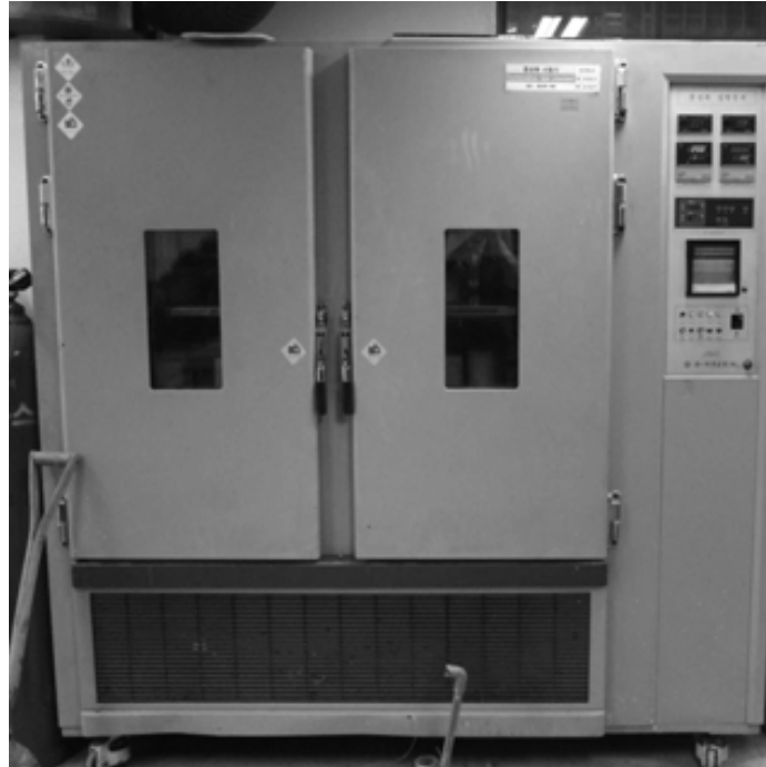
Figure 4. Creep test setup.
