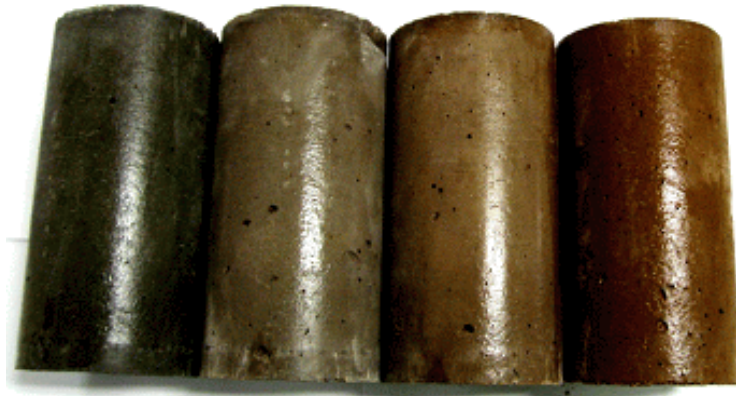
Figure 2. 100 mm × 200 mm Hwangtoh and slag cement concrete cylindrical specimens.
