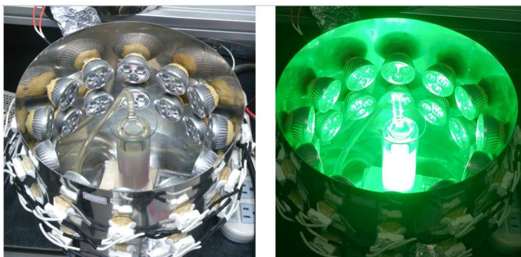
Figure 12. The setup for the temperature-controlled photochemical reaction with green LEDs.
