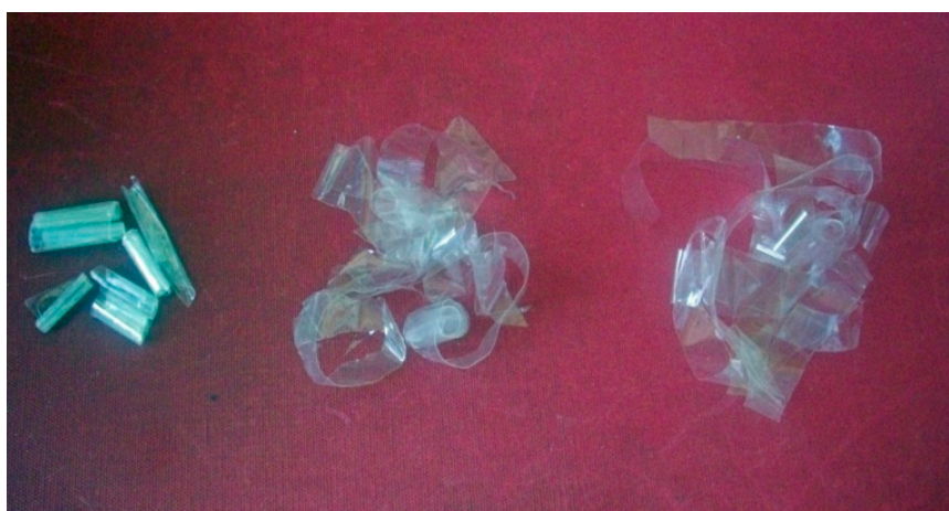
Figure 4. PE/Whey/PET films after treatment with 4% Terg-a-zyme for 1, 2, and 4 h.
