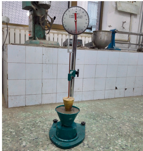
Figure 3. Consistency test of mortars.
