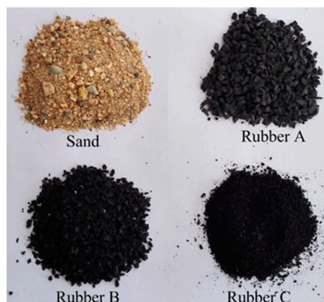
Figure 1. Fine aggregates: Sand, Rubber A, Rubber B, and Rubber C.
