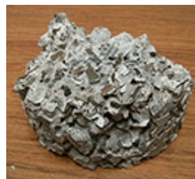
Figure 13. A large intact piece of pervious concrete broken off from the bulk of the sample while being tested with the 24 h cycle saturated with 50 mm of solution.
