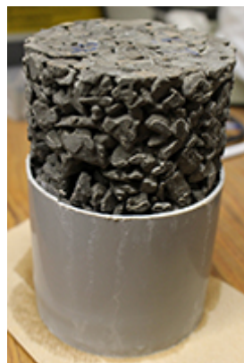
Figure 4. Pervious concrete cylinder partially saturated using a mould with a height of 75 mm.
