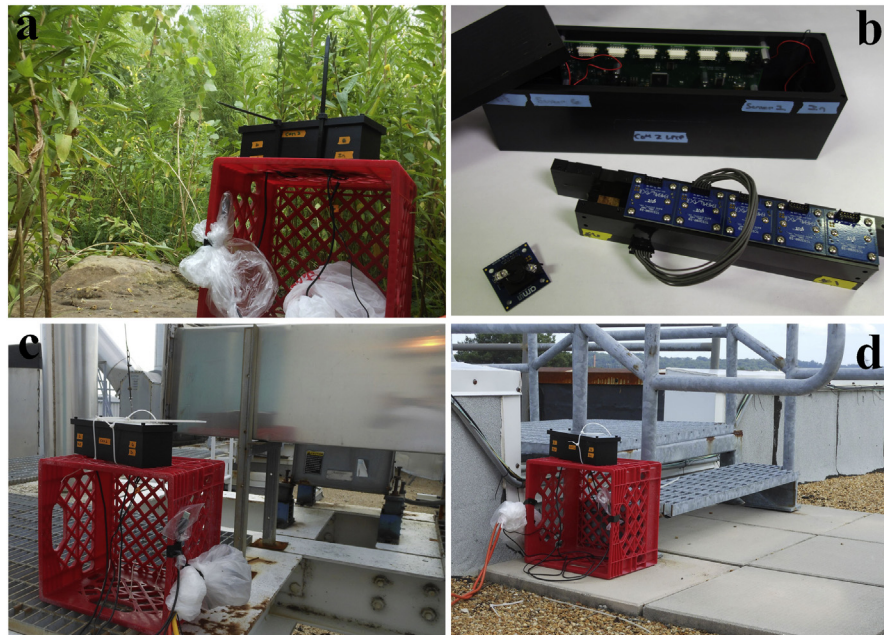
Fig. 1. Photographs of the prototype devices: (a) device in outdoor, simulated forest environment; (b) detail of device components; (c) device on roof top at ~18 m; (d) device on roof top at ~11 m.
