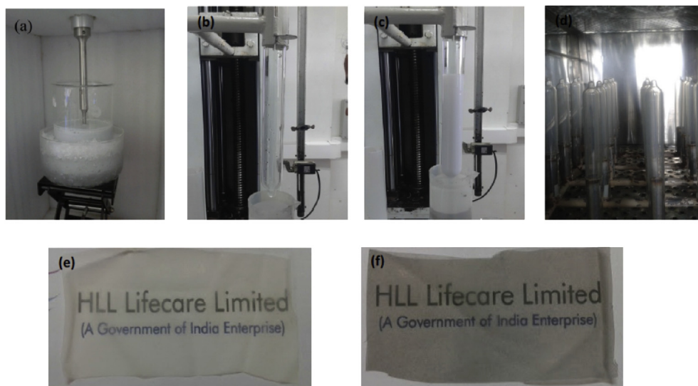
Fig. 2. Production process of graphene reinforced NR latex nanocomposites (a) Sonication followed by (b) first dipping of the mould, (c) second dipping and finally (d) vulcanization in hot air oven. The produced NR latex control sample (e) was kept on a printed paper along with graphene-NR latex nanocomposites thin films (1.5 phr) (f) to test the transparency of both samples. (A colour version of this figure can be viewed online.)
