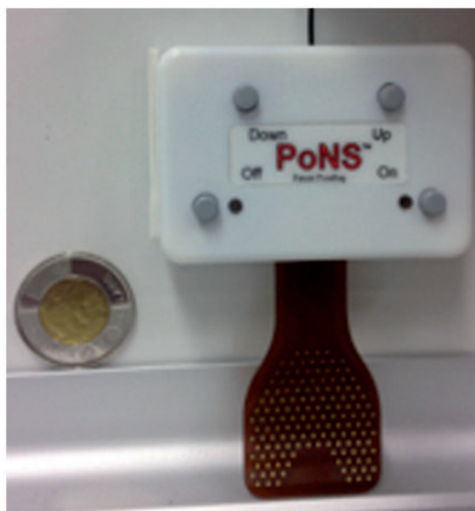
Figure 1. The relative size of the Portable Neuromodulation Stimulator as compared to a Canadian two-dollar coin.
