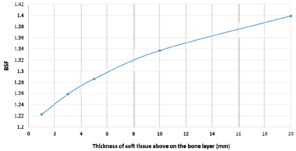
Fig. 7. Backscatter factors as a function of water thickness on the entrance surface above the bone layer calculated by convolution of the backscatter PSF for the 20 cm square field sizes.
