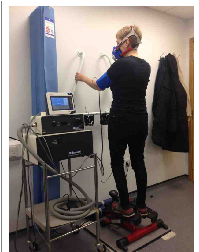
FIGURE 1 | Example set-up for the 6-min stepper test including blood pressure monitor and gas analysis mask.
